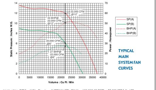
A OMC-1736 RPM = 1631 ; Density = 0.0728 Lb/CF ; Width = 100.00% 50 BHP at 22,000 CFM @ -12" B OMC-1736 RPM = 1321 ; Density = 0.0739 Lb/CF ; Width = 100.00% 27 BHP at 22,000 CFM @ -6"
